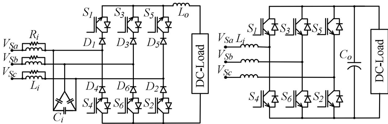
Fig.2a PWM Current Source Converter      Fig.2b PWM Voltage Source Converter
