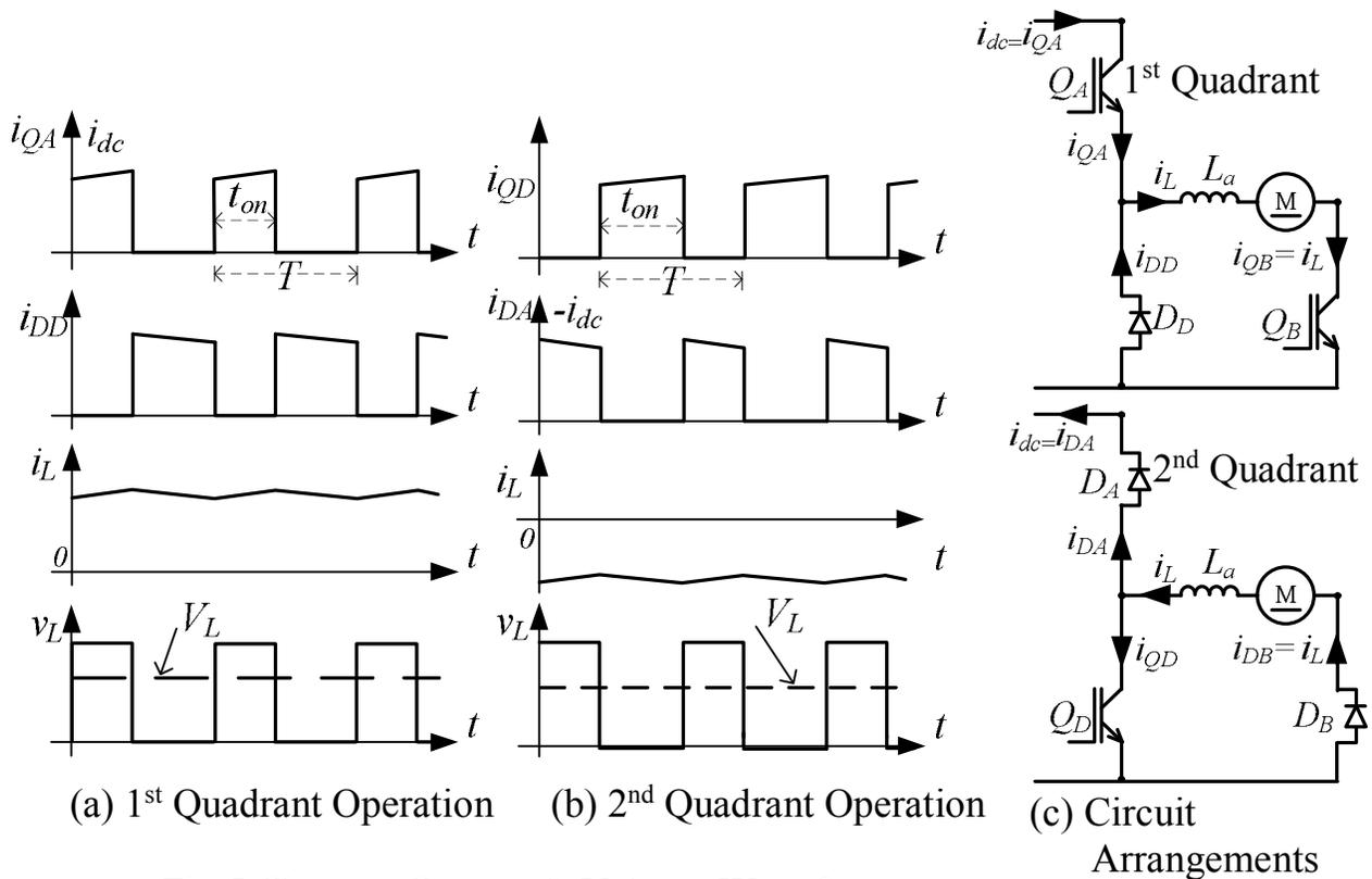
Fig.5 Chopper Current & Voltage Waveforms
