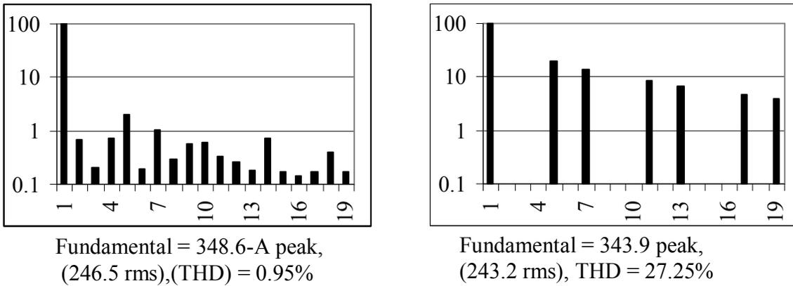
Fig.9e Comparison of Harmonic Spectrum of line Current
