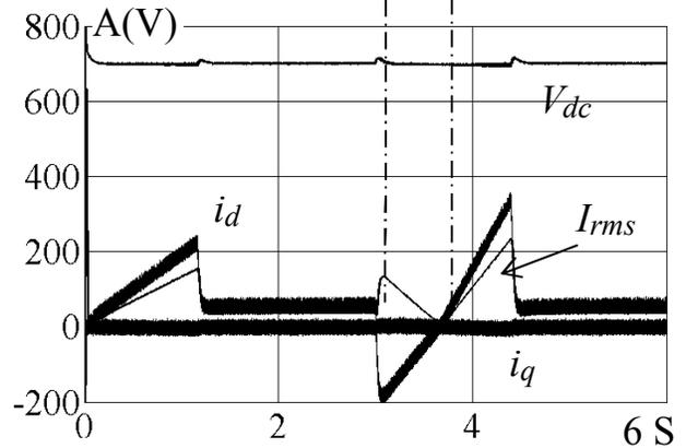
Fig. 8b Converter VOC Response for a  $\pm 1.0$  pu ramp speed reference.
