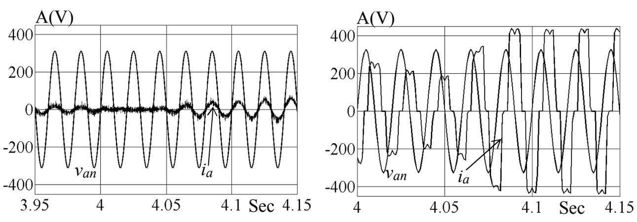
Fig.9c Supply Voltage & Line Current During Speed Reversal
