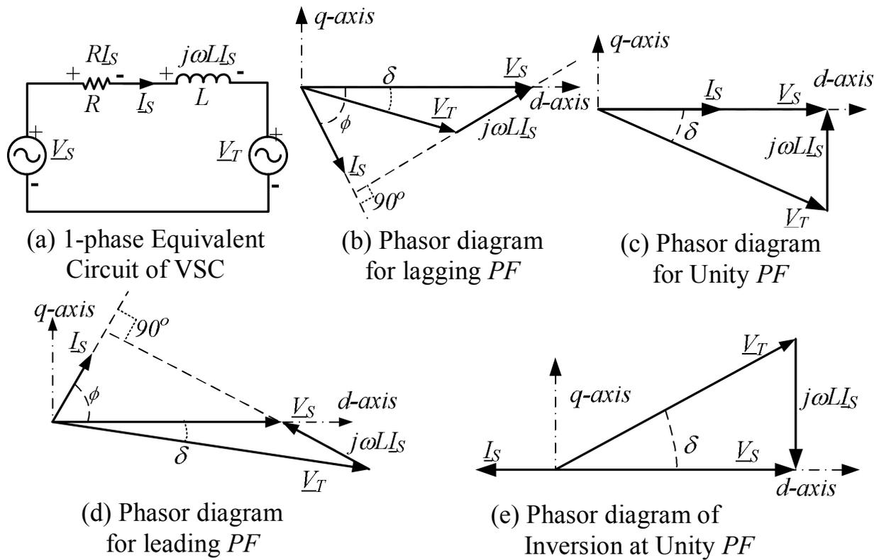
Fig.4 Clarifications of Different Modes of Operations VSC
