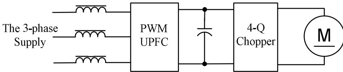
Fig.1 Simple Block diagram of The Suggested DC Motor Drive
