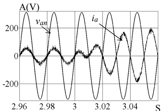
Fig. 8c Supply Current during Speed Reversal
