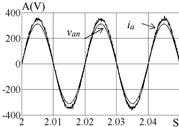
Fig. 7c Steady-State  $i/v$  of Supply at Full Load
