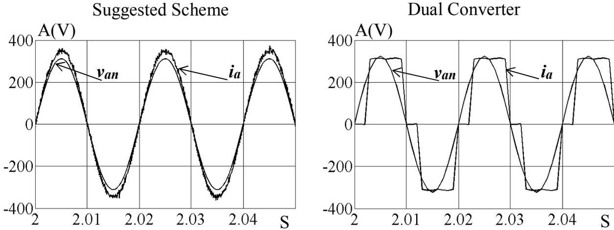
Fig.9d Comparison of Supply Current During Steady State Speed
