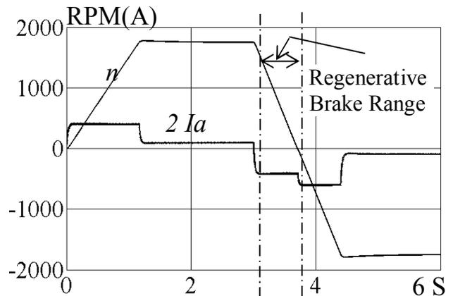
Fig. 8a Speed and Current Response for a ramp speed reference.
