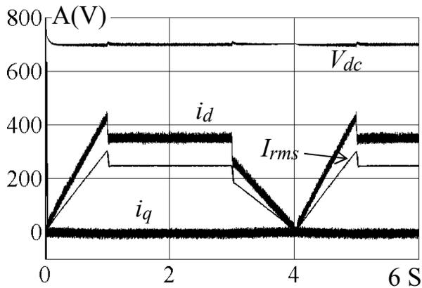
Fig. 7b Converter VOC Response for a  $\pm 1.0$  pu ramp speed reference.
