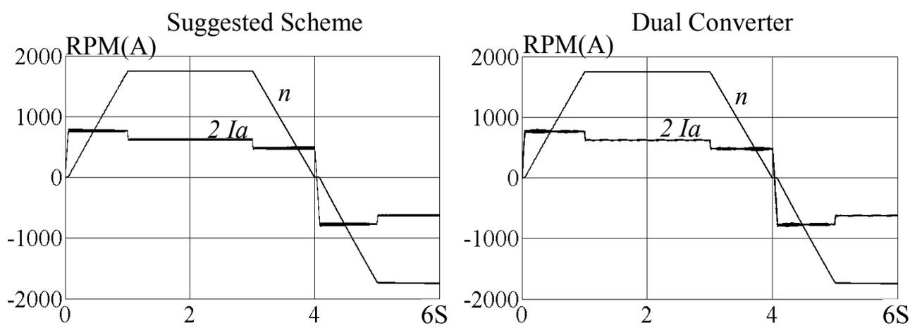
Fig.9a Comparison of Speed Response.
