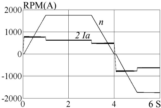
Fig. 7a Speed and Current Response for a ramp speed reference.
