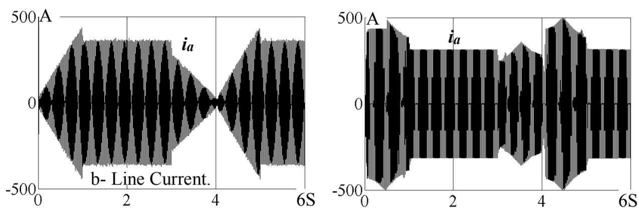
Fig.9b Comparison of envelope of the Line Current.
