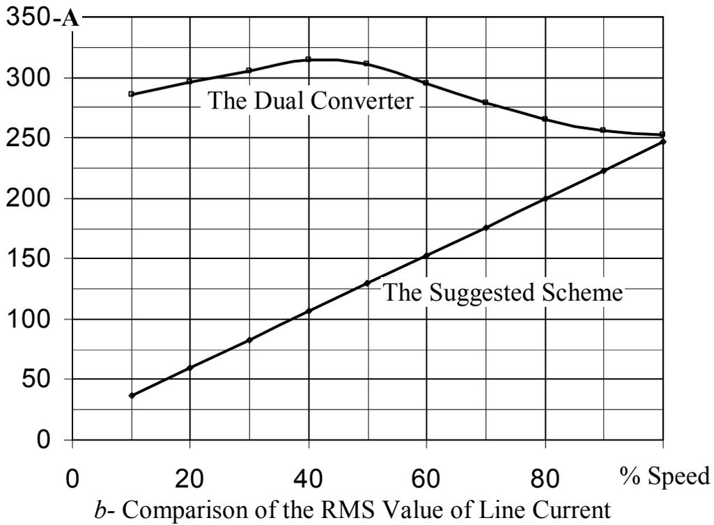
Fig.10 Comparison of Performance of the Suggested Scheme and the Dual Converter over the Full Range of Speed.
